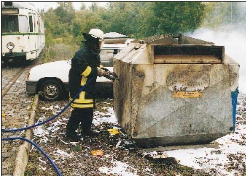
The homemade lance nozzle being used on a paper-recycling container at Wattenscheid.
